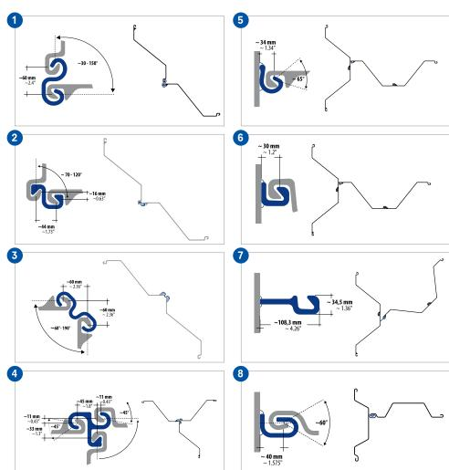
We can also supply the sheet pile sections with the required angle in them.
